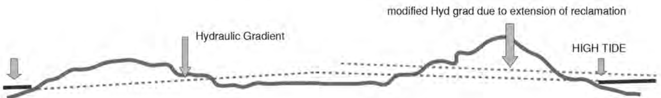
Figure 6 :Storm water hydraulic line at high tide after reclamation
