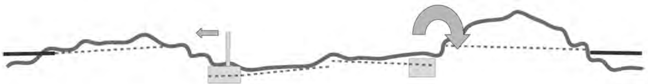
Figure 7 :storm water disposal through pumping
